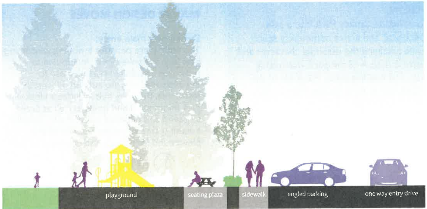
FIGURE 3.3: Section “A” through main entry hub; the plaza and playground are easily accessed from the parking area but are visually screened with ornamental plantings
